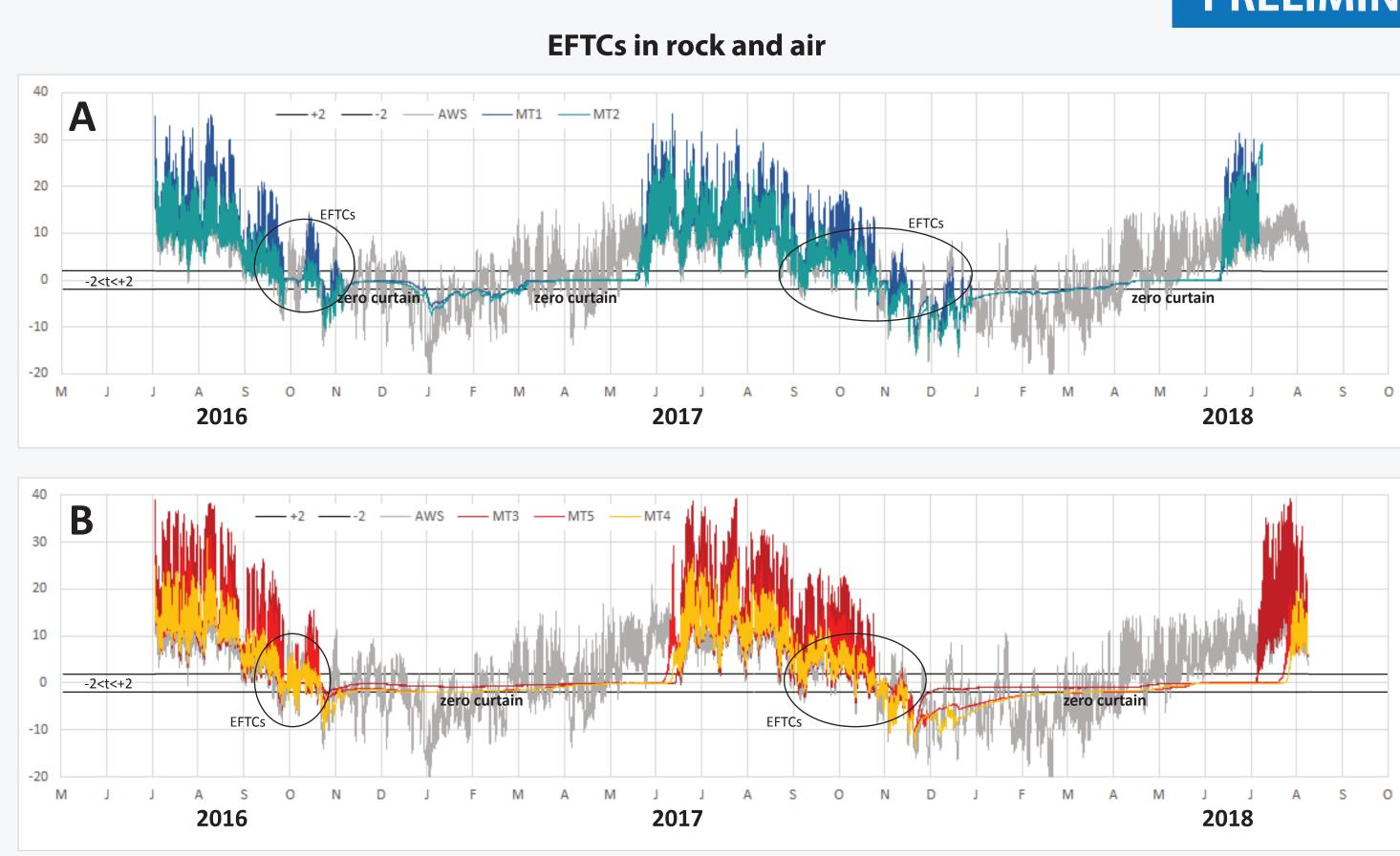
Analysing rock temperature trend in the measurement period some observation can be done: - the insulating effect of the snow cover in winter and spring ("zero curtain", i.e. nearly constant temperature close to the freezing point) is well
